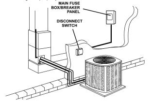
NOTE — Units are approved for use only with copper conductors. Ground unit at disconnect switch or to an earth ground.
